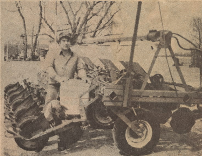
Tom Barthel, above, with his no-till corn planter. Barthel has been using this planter with various degrees of tillage for several years to reduce wind erosion and save time. Barthel farms are northeast of Becker.
